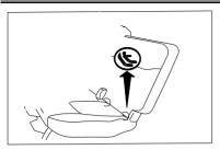
ISOFIX Child Seat Anchorage Your car is equipped with special anchor point for the child safety seat with ISOFIX child seat anchorage. (on rear seat)
