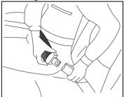
Press down the button of seat belt lock catch to enable the seat belt to goes back automatically.
